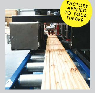
For a quicker and more effective service we recommend sending us your timber before softwood treatment as GripDeck® anti-slip inserts bond best to untreated timber. Our GripDeck® inserts will not be harmed by the timber treatment process after they have been bonded to your timber.
